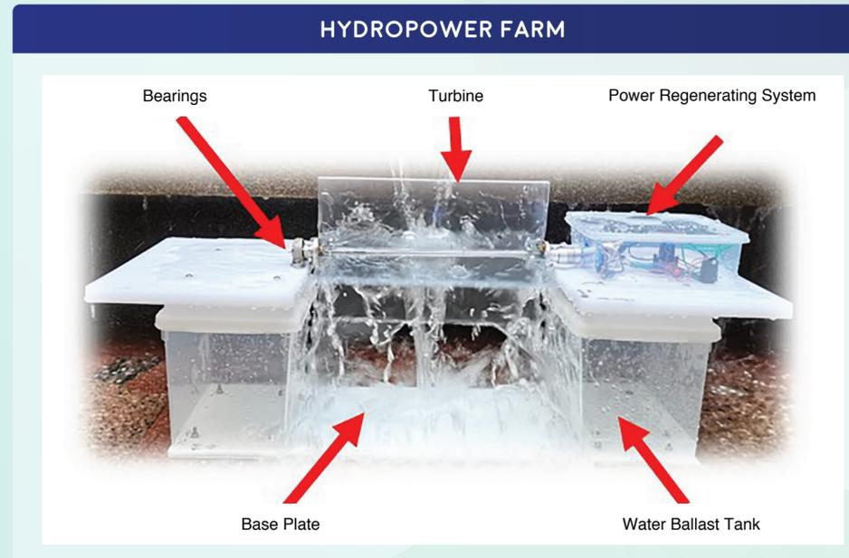
PROTOTYPE PLACED IN THE FOUNTAIN AT ITE CC THAT USES THE FLOW OF WATER TO GENERATE ELECTRICITY. THE TURBINE WILL LIGHT UP THE LEDS WHEN POWER IS GENERATED.
